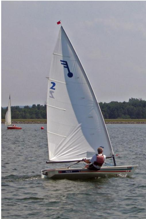
The Force 5 is a powerful single-handed racing dinghy. Although one person races the boat, the cockpit is large enough to accommodate two people and provide ample day sailing enjoyment. This 14' craft has a 91 square-foot mainsail, rolled deck and an adjustable rig. It is easily car topped. The class association website is [www.force5.us](http://www.force5.us).
