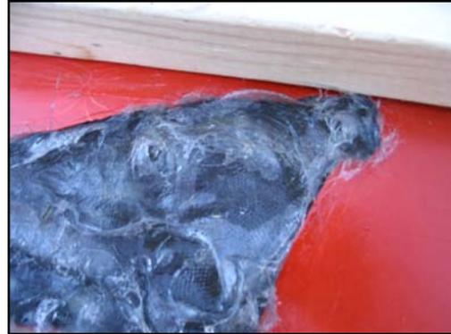
In about four hours, this will give you a solid piece of fiberglass. Then, peel back the foam board from fiberglass.
